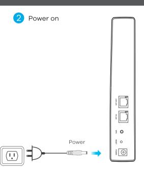
Blue Blinking - System is booting On - System is ready.
