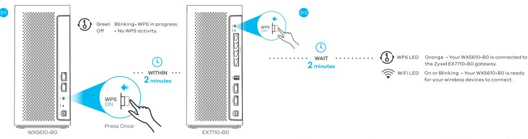
Press the **WPS** button once, the WX5610-B0 **WPS** LED (3) blinks green. **Within Two** minutes, press the **WPS** button on your Zyxel EX7710-B0 gateway. If the WX5610-B0 **WPS** LED (3) turns red, do the process again.
