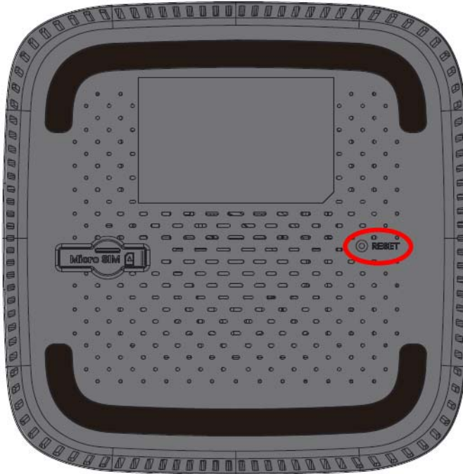
Figure 39 NR5103EV2 / NR5103EV3 Reset Button
