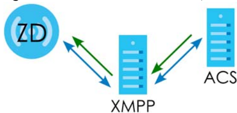
Figure 192 XMPP Connection Request
