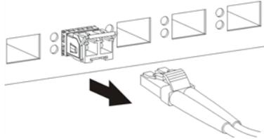
**Figure 7** Opening the Transceiver's Latch Example
