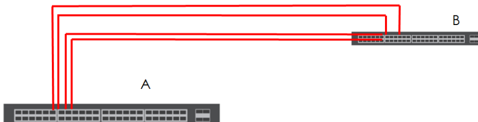
Figure 93 Trunking Example - Physical Connections
