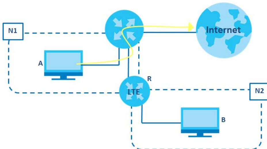
You need to specify a static routing rule on the Zyxel Device to specify **R** as the router in charge of forwarding traffic to **N2**. In this case, the Zyxel Device routes traffic from **A** to **R** and then **R** routes the traffic to **B**.
