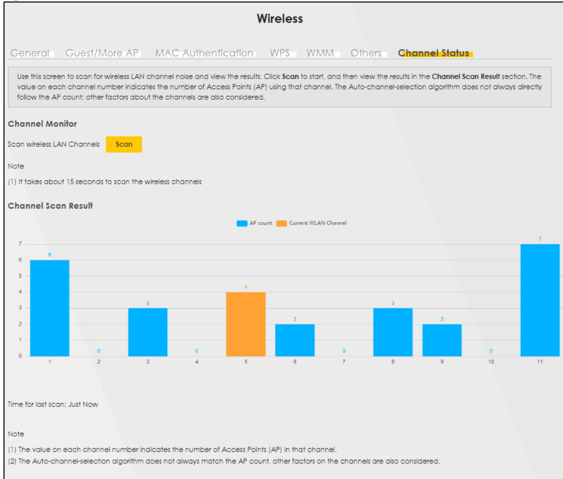
Figure 111 Network Setting &gt; Wireless &gt; Channel Status
