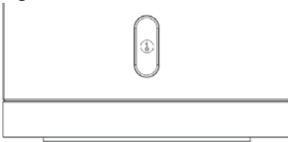
Figure 21 WPS and WiFi On /Off Button on the Front Side of the Zyxel Device (EE3301-00)
