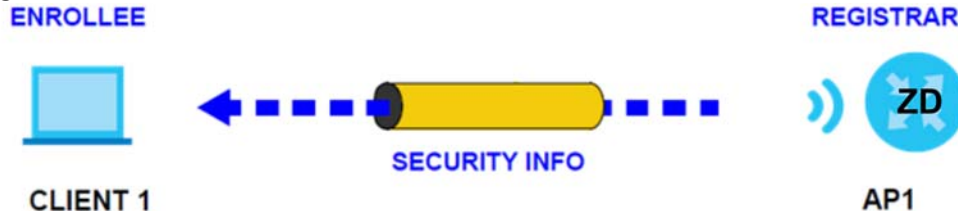
Figure 111 WPS: Example Network Step 1
